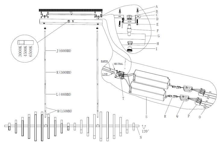
NOTE: Do not rotate the arm more than 60° as this may damage the knuckle joint or the internal wiring.
