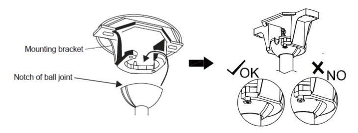
4. Slide the Canopy up into place over the ceiling mounting bracket. The two screws on the mounting bracket face should slip through the key hole slots in the canopy face. Rotate the ceiling canopy slightly to place the screw heads in the small end of the key hole slots. Tighten both screws.
