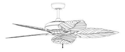
2. Align the holes of light kit and the holes on the bottom of motor housing cover, slide the light kit clockwise with 3 screws to secure.
